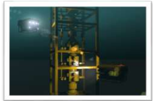
Figure 1: The ROVs can monitor a BOP
